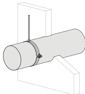
2. Provide suspension where necessary in accordance with the instructions of the duct manufacturer.
