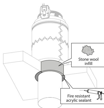
5. Insulate the duct with stone wool (min. El 60 S) according to the stone wool manufacturer's instructions.
