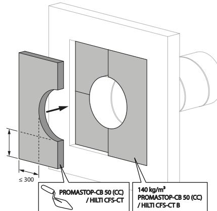
2. The fire batt may be replaced by a similar type of fire batt with at least the same fire reaction class, density and thickness (tested according to EN 1366-3).
