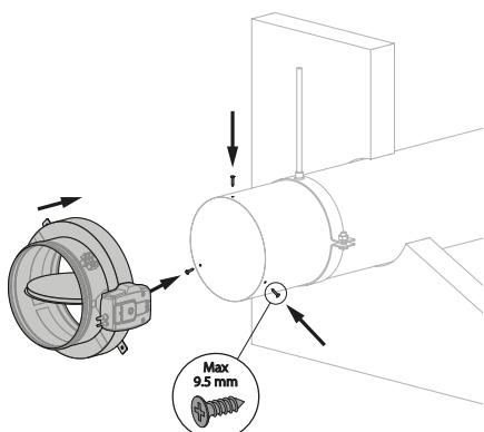
3. Attention: Make sure that the movement of the damper blade is not impeded by the screws.
