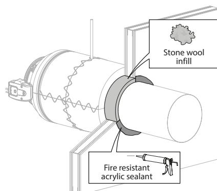
5. Insulate the duct with stone wool (min. El 60 S) according to the stone wool manufacturer's instructions.
