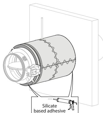
4. Insulate the duct with stone wool (min. EI 60 S) according to the stone wool manufacturer's instructions.
