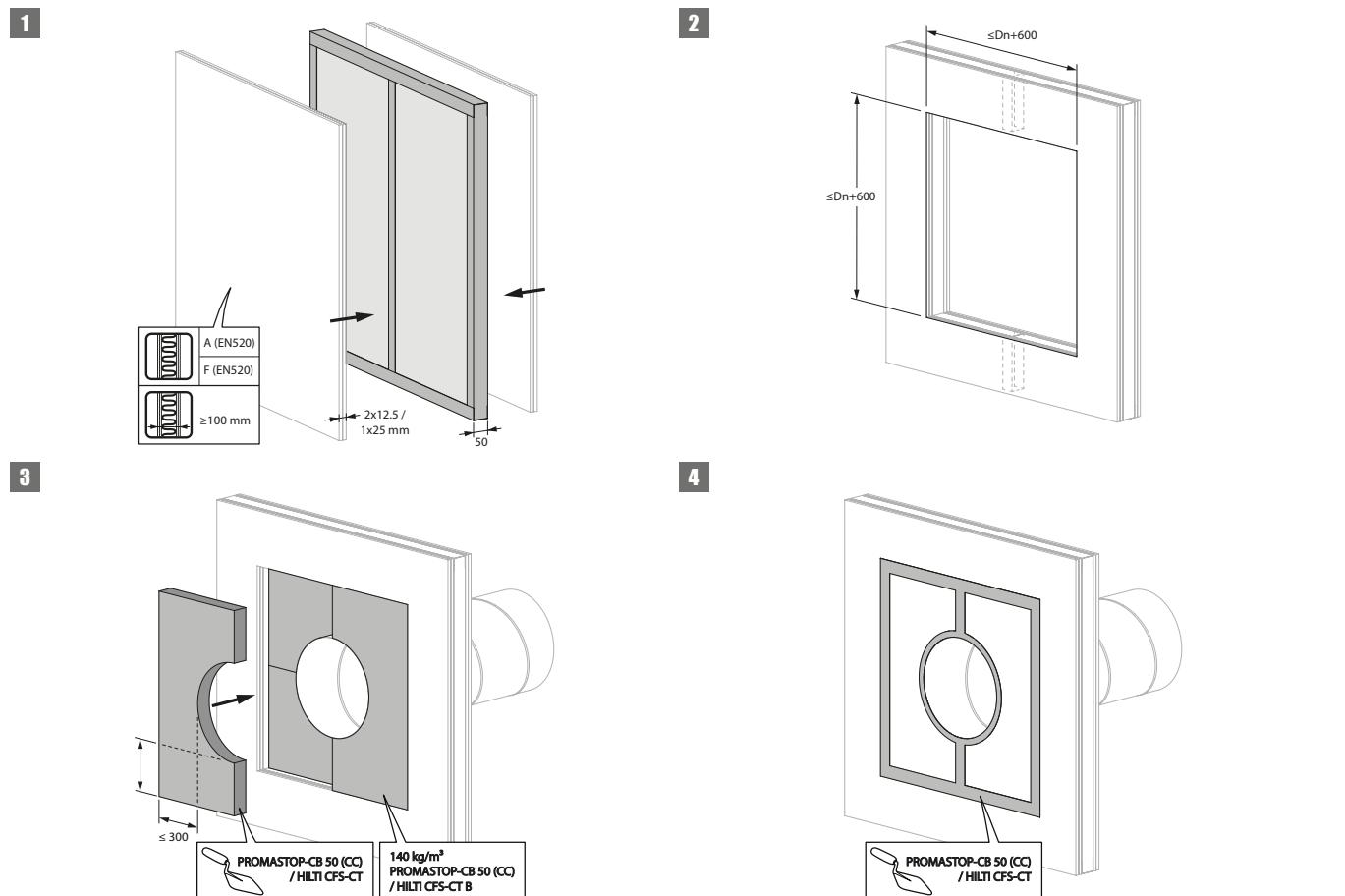
3. The fire batt may be replaced by a similar type of fire batt with at least the same fire reaction class, density and thickness (tested according to EN 1366-3).
