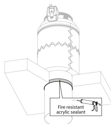
5. Insulate the duct with stone wool (min. EI 60 S) according to the stone wool manufacturer's instructions.
