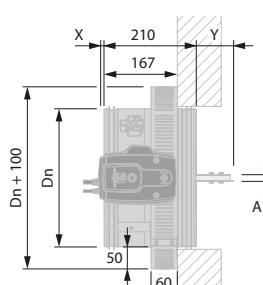
Exceeding blade: X = on the mechanism side, Y = on the wall side
