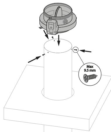
4. Attention: Make sure that the movement of the damper blade is not impeded by the screws.
