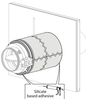
5. Insulate the duct with stone wool (min. EI 60 S) according to the stone wool manufacturer's instructions.
