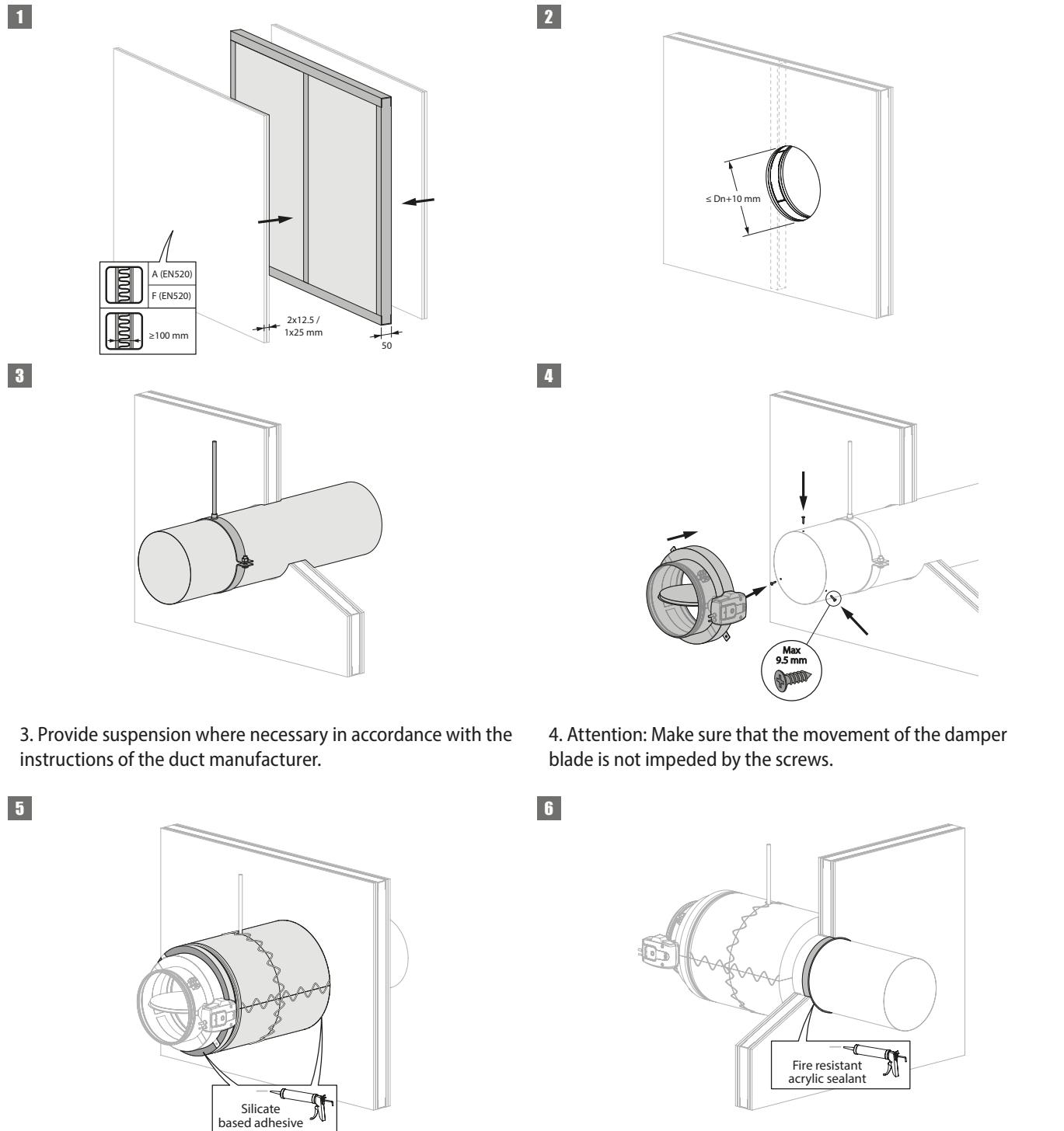
3. Provide suspension where necessary in accordance with the instructions of the duct manufacturer.
